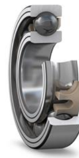
Figure 11. Special hybrid deep groove ball bearing for cryogenic pumps, with a special PEEK cage and nitrogen steel rings according SKF VC4444 specification.
