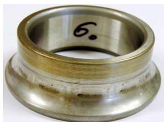
Figure 15. High-nitrogen stainless steel inner ring in the same H 2 -rich application as in Figure 14, after about 8000 hours [17].
