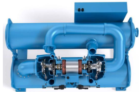
Figure 8. Illustration of a chiller with a sectional view of the two stage centrifugal compressor using PRL bearing technology [4].
